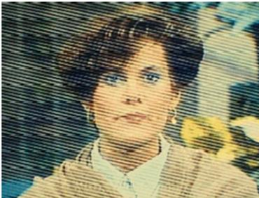
Picture 5: Ham/CB Transmitter Interference
