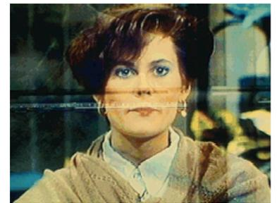
Picture 4: Co-channel Interference
