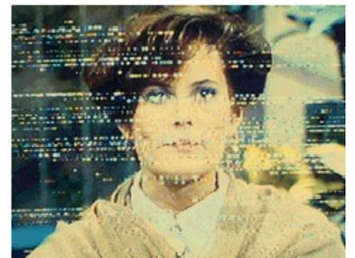
Picture 6: Electrical Interference -- very noisy (hair dryer)
