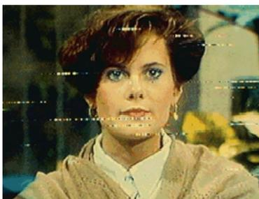
Picture 7: Electrical Interference -- low noise
